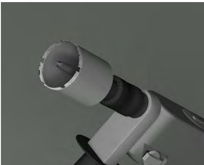
Diamond-tipped core drill
