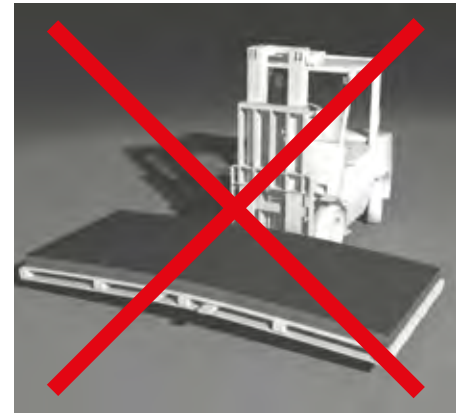
Improper forklift transport
